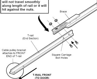
• Position the cable pulley bracket on the front end of the T-rail as shown. Fasten securely with the hardware.
